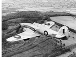
A Royal Air Force Hawker Hurricane Mark IV fighter-bomber armed with RP-3 rockets in flight, August 1945: http://schools-wikipedia.org/images/87/8754.jpg.htm Expired Crown Copyright image no. MH4943 from the Imperial War Museum collections
